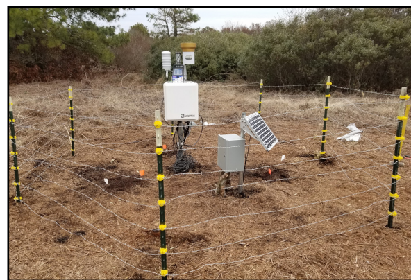
Fig. 1. Soil moisture monitoring station in the Pocosin Lakes National Wildlife Refuge in northeastern North Carolina
