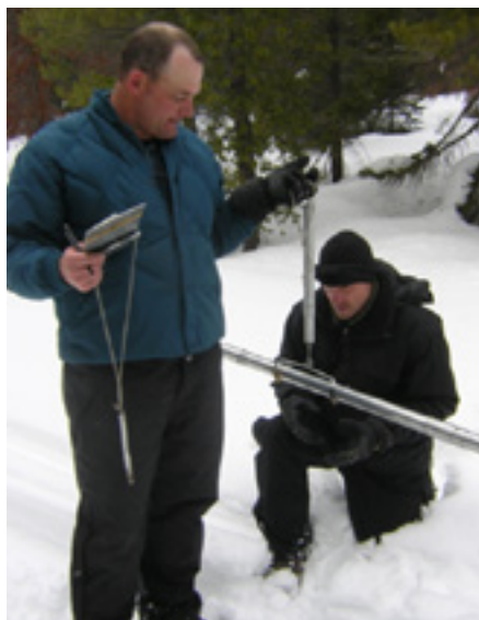
Chad Pickett and Kevin Pantle of the Wyoming State Engineer's Office conduct snowpack reading at the Haskins Creek Snow Course in Wyoming's Sierra Madre Mountains. Photo by Matt Hoobler, Wyoming SEO
