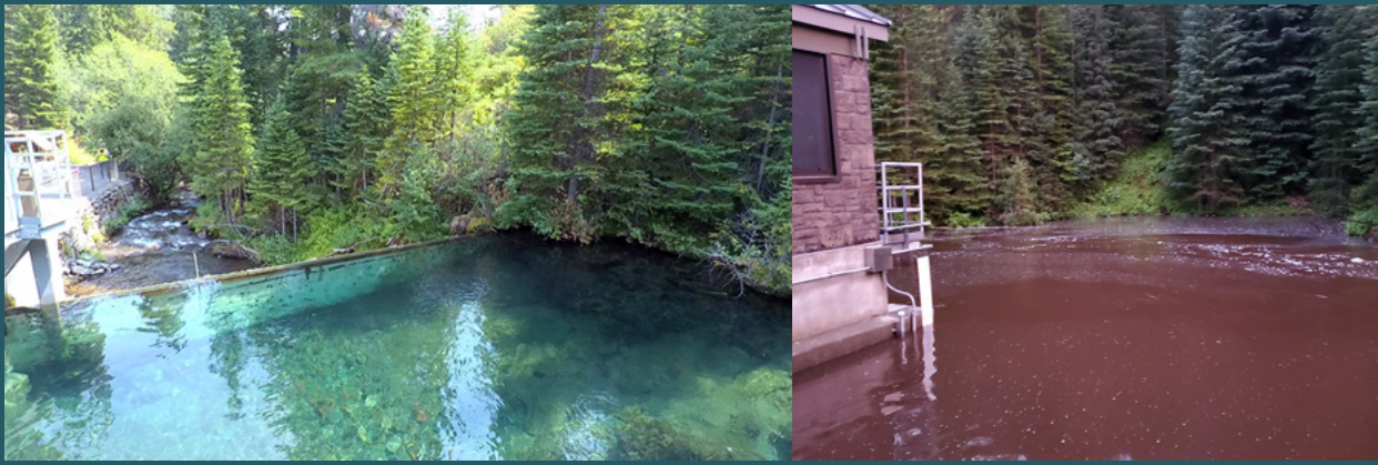
Figure 15: The image on the left shows typical turbidity levels and the image on the right shows the high turbidity on August 5, 2020 associated with a major thunderstorm in the Tumalo Creek Watershed municipal water supply for Bend, Oregon (City of Bend).
