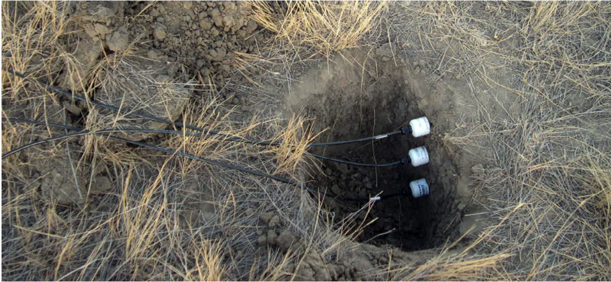
USCRN soil moisture station installation, Fort Peck Tribes Reservation, Montana. Credit: Tilden Meyers
