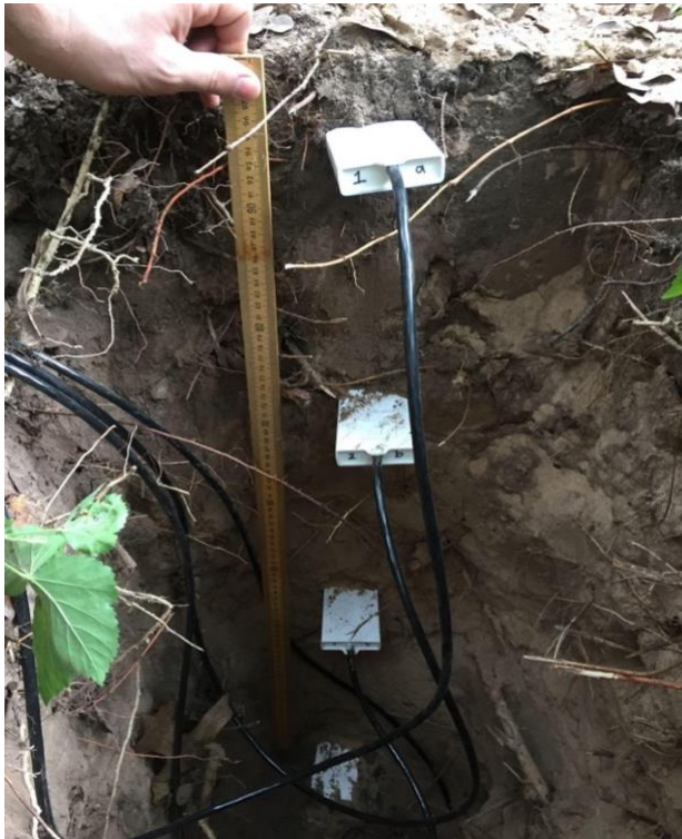
Figure 2. Photo of soil profile and soil moisture sensors installed to a depth of 1.0 m. Photo Credit: Briana Wyatt.
